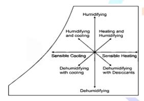
The process in which the moisture or water vapor or the humidity is removed from the air keeping its dry bulb (DB) temperature constant and reduces the humidity ratio is called as the dehumidification process.
